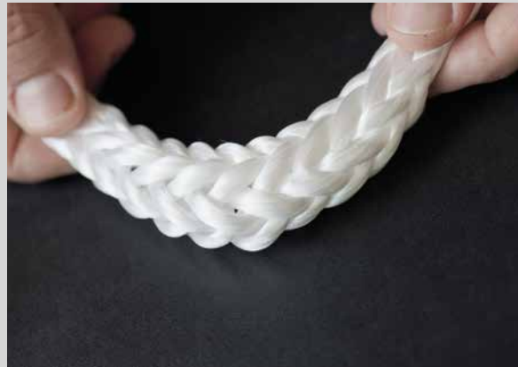
Single braid Dyneema® without HPS treatment: the braid is soft and "airy".
