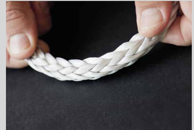
The braid after the HPS treatment: the fibers are oriented and the rope is more rigid and compact.
