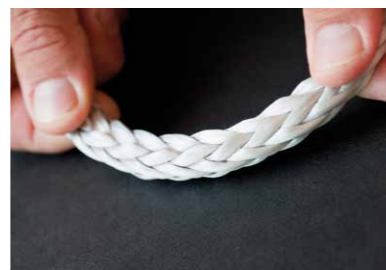
The braid after the HPS treatment: the fibers are oriented and the rope is more rigid and compact.
