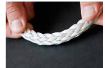
The braid after the HPS treatment: the fibers are oriented and the rope is more rigid and compact.
